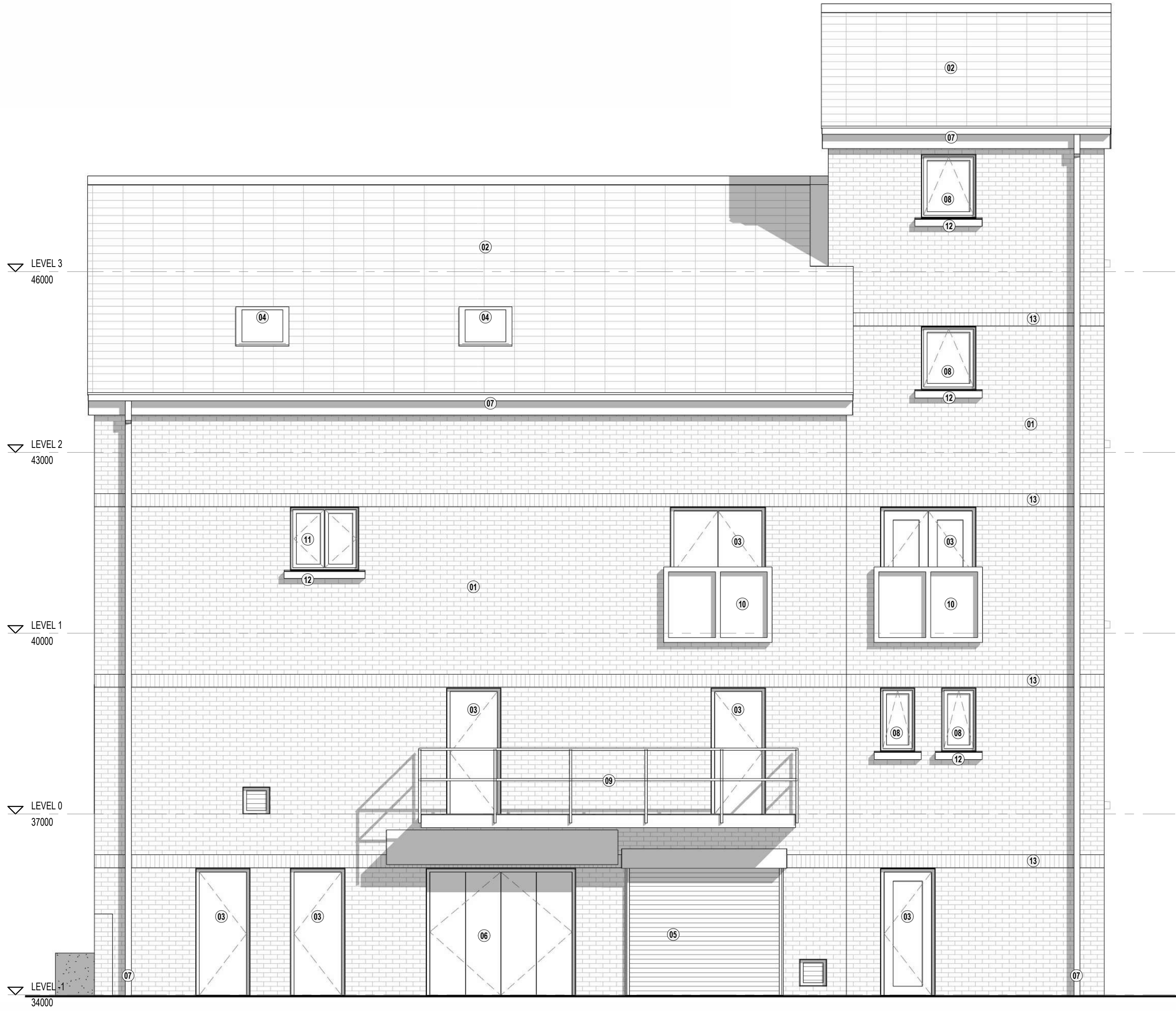
NORTH FACING ELEVATION 1 : 50
